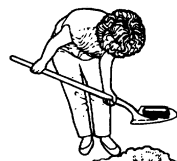
Figure 1b. Use a hand trowel, shovel or other garden tool. Trim out soil of uniform thickness to the recommended depth.
